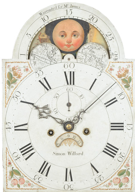
A Birmingham painted dial by James Wilson (d. 1809). The Wilson firm is credited with “making dials in imitation of enamel” and the introduction of the “false plate” as a means to streamline the mounting of dials to movements.
