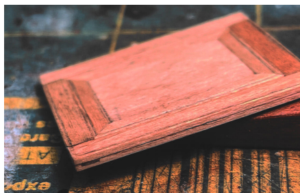
Photos 24a, 24b. The author's door constructed with half lap joints, AP
